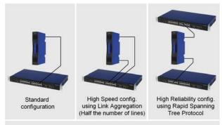
Different IP DSLAM Configurations
